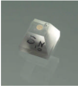
Fig. 7 Acrylic sample holder for small amounts, used for GADDS and \mu -XRF.
