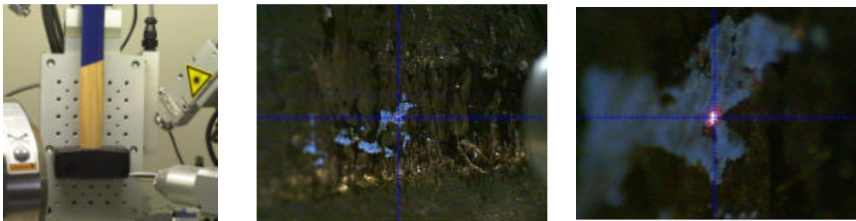
Fig. 21 Examination of small contact traces on a hammer, adjustment the blue contact trace and measured area.
