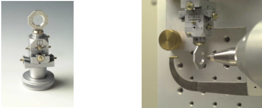
Fig. 15 Preparation of small amounts of powder on a sample holder with a 3 \mu\text{m} sheet of Mylar.
