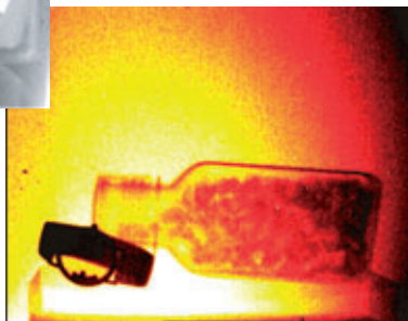
Pseudo-colour definition according to object density
